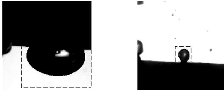
Fig. 2. Views of vapor bubbles before they detach from the lower part of the cylinder (left) and the upper part (right). The spatial scale is the same in both photographs. The dashed lines indicate the Region Of Interest over which the bubbles are detected and the bold lines indicate the detected bubble boundaries.
